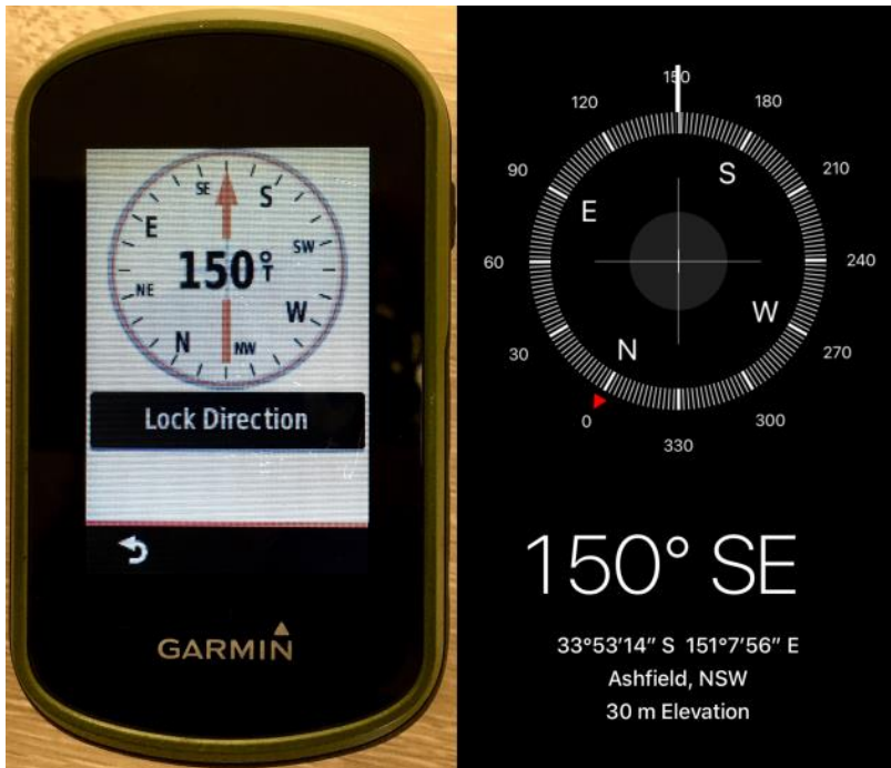
Figure 2: A handheld GPS unit such as the Garmin etrex touch 35 (on the left) or the iOS compass application (right) can be used to determine the longitude and latitude of the recording location and the absolute bearing of the camera.
